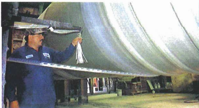
Tank ribs are constructed on a rotating steel mold during the automated manufacturing process. Our precision technology results in a more consistent tank thickness and composition than competitive products.
